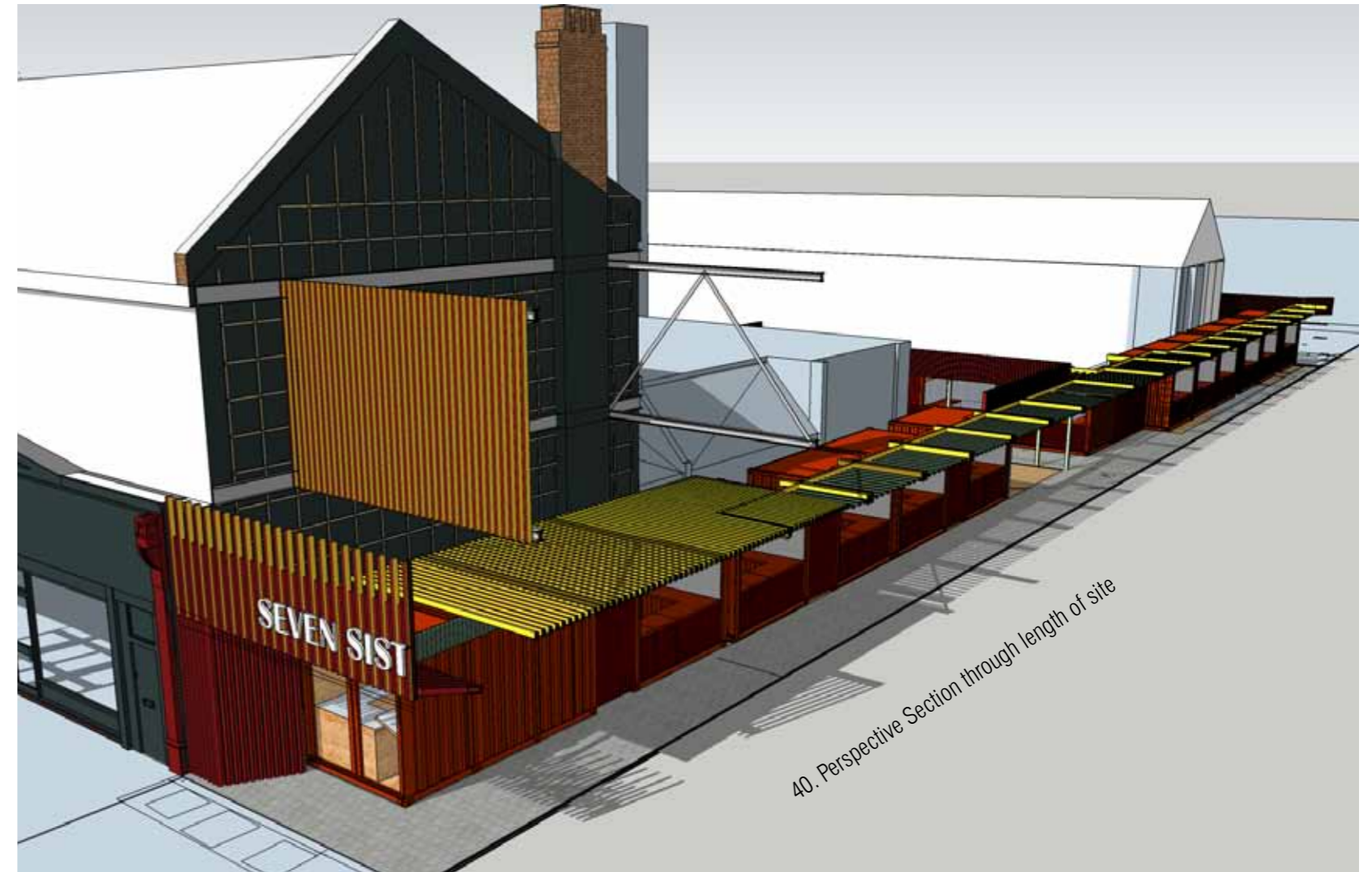
43. Cut-away perspective section of 3d model, view looking South-westwards from the High Road. (Temporary indoor market, left)
